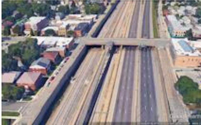
**IDOT's Model of the Proposed Harlem Avenue Interchange showing the horizontal beams connecting the eastbound and westbound ramps**
